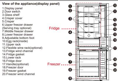
**Note:** Due to unceasing modification of our products, your retrigerator may be slightly different from this instruction manual, but its functions and using methods remain the same. To get more space in the freezer you can remove drawers (except the bottomdrawer in freezer!) .To get the best energy of this product please place
