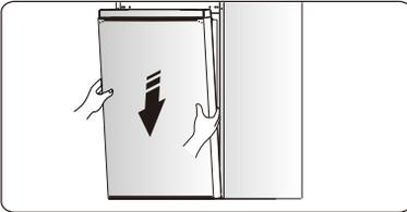
13. Slot the lower door onto the bottom hinge pin and hold in position. Turn the middle hinge by 180°, change the washer on the axis to the lower side, adjust the middle hinge to the appropriate position and then install it ensuring the lower door is secured in place.
