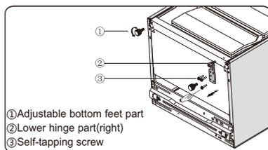
9. Remove part ① from the lower hinge part(right), loose out the lower hinge pin, change it to the reverse hole site, and then tighten into position, then install part ① on the lower hinge pin.
