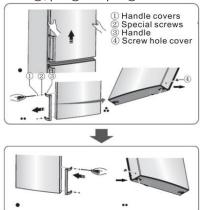
**Warning!** When changing the side at which the door opens, the appliance must not be connected to the mains. Remove plug from the mains beforehand.
