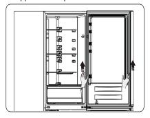
4.Loose screw ③ and take down part ② and part ①, Install replacement door stopper-left ④ (provided in the plastic bag) and part ②(stop block) to the left side with screw③. Keep part ① with the appliance for future reference.
