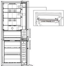
2.Remove part①, then take down part② from the top right side of refrigerator. Unscrew screws③ by a 8mm socket driver or a spanner, and remove hinge④. Please hold upper door by hand when installing. Use a putty knife or thin-blade screwdriver to lever part⑤ which is at the top left corner of the refrigerator.
