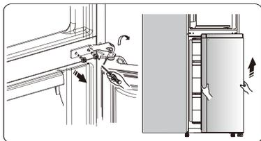
6. Place the lower door on a smooth surface with its panel upwards. Loose screw ③ and take down part ① and part ②, then Install door stopper-left ④ (provided in the plastic bag) and left part ② and screw ③ to the left side and tighten them securely. Keep part ① with the appliance for future reference.
