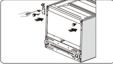
12. Transfer the lower door to the property position, adjust the lower hinge part, make the hinge axis into the lower hole of the lower door, then tight the bolts.
