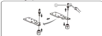
10. Change screw hole covers on lower cover plate from left to right (as shown in figure below).
