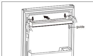
Firstly hold the two side of the door shelf tightly, fit the door shelf along the guides on the door, then push it down to the right place.
