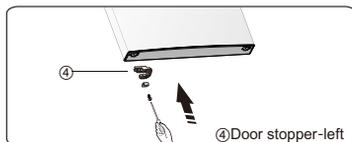
7. Change screw and screw hole covers on middle cover plate from left to right (as shown in figure below).
