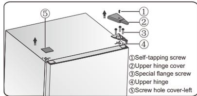
3. Remove the upper door from the middle hinge by carefully lifting the door straight up. Then place the upper door on a smooth surface with its upper cover upwards.
