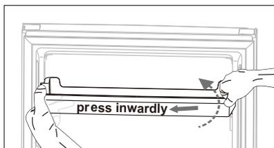
Hold one side of the door shelf, press the opposite side inwardly by the other hand, then lift up the door rack. When the slot of the door rack has been detached from the guide on the door, remove the rack upward obliquely.
