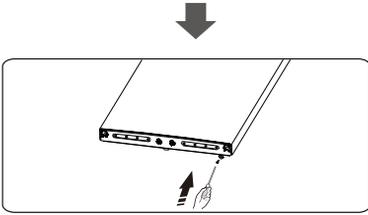
6. Lay the refrigerator on soft foam packaging or similar material. Remove both adjustable bottom feet parts, and the lower hinge part by unscrewing the special flange self-tapping screws.
