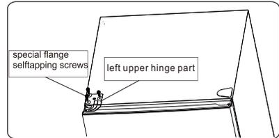
3. Remove the upper hinge axis, transfer it to reversed side and tighten securely, then put it in a safe place.
