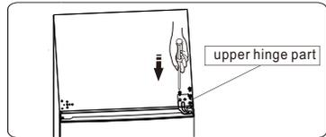
10. Install the screw hole on the top left corner of the refrigerator. Install the upper hinge (which is in the plastic bag) on the right corner. Put the other upper hinge cover into the plastic bag.
