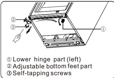
7. Replace the lower hinge part to the right side and fixing it with the special flange self-tapping screws. Replace the adjustable bottom feet part to another side and fixing it.
