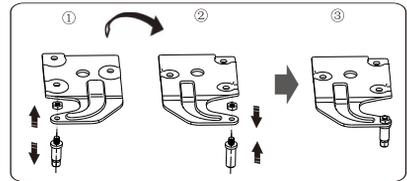
4. Remove the door from the lower hinge.
