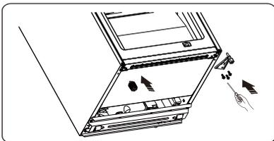
8. Transfer the door to the properly position, adjust the lower hinge part, make the hinge axis into the lower hole of the door.
