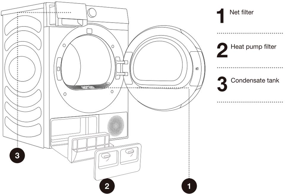
**⚠** The dryer may never be operated without the filters in place or with damaged filters, as excessive amount of accumulated fibres from the fabric could cause malfunction or failure of the dryer.
