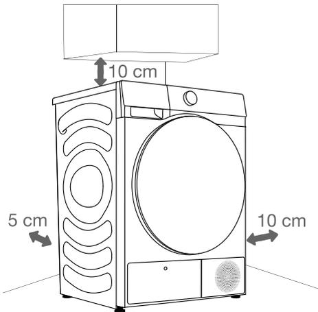
⚠ The dryer may not be in contact with a wall or adjacent furniture. For optimum dryer operation, we recommend observing the clearance from the walls as indicated in the figure. In case of failure to heed the required minimum clearance, the dryer may overheat.
