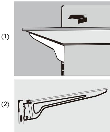
2. To reinstall a shelf, gently slide the shelf back into the refrigerator compartment, and lower the shelf onto the rail support.
