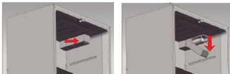
2. Pull the water filter down wards and turn it about 90° counter-clockwise to take it out. When the filter is disassembled, pay attention to keep the filter head upward tilted to avoid water leaking from the front filter part. And the dropped water in the cover should be cleaned immediately.
