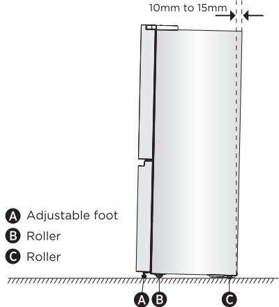
**NOTE:** Having someone push against the top of the refrigerator takes some weight off the leveling feet. This makes it easier to turn the feet. Rotate the adjustable feet clockwise to raise or counter-clockwise to lower your refrigerator. To make sure that the doors close automatically, tilt the top of your refrigerator backward about 10mm to 15mm. If necessary, use a spanner wrench to adjust the feet.
