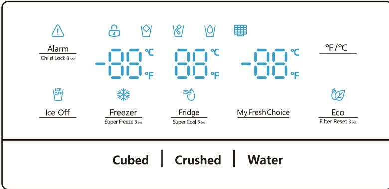
The display will illuminate when the refrigerator is first plugged in. However, the lights will automatically turn off after 60 seconds.
