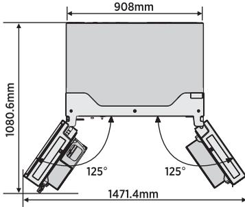
The four doors can be opened and closed either separately or together.
