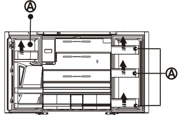
To remove the door baskets (B), take the right side of the baskets out by lifting it at an angle along the guide, and then take the left side out by pulling it from the door.
