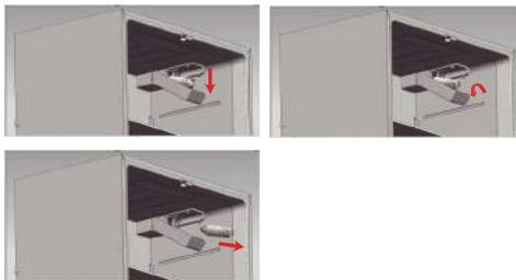
3. Insert the new water filter into the hole, and at the same time turn it about 90° clockwise until it stops.
