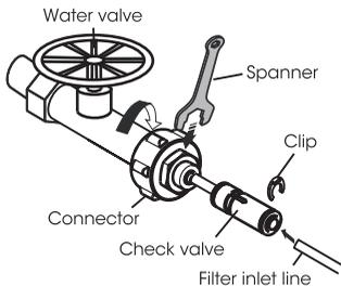
To prevent the clips loose, use the valve seat to hold it. Then use the screw to hold the valve seat with Philips(+) screwdriver.
