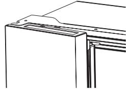
**NOTE:** Before closing the left-hand door, make sure the mullion is folded inward. If the mullion is pulled outward it may become damaged when you try to close the door.
