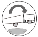
1. Take out the water box horizontally to avoid spllover of condensate water.
