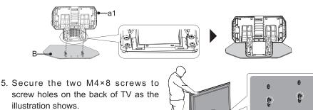
6. Hang the assembled Part a1 and Part B to the two M4×8 screws you have secured to the TV, then secure the assembled part to TV with four M5×16 screws. You can adjust the height of base stand to H1 or H2. For H1, secure screws to four hole 1.
