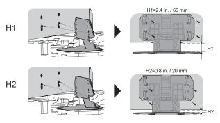
**NOTE:** Keep the television vertically when you remove the base stand. If you place the TV face down, the base stand may fall down on your feet while removing it.
