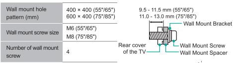
We do not recommend hanging the TV on a slanted wall, and when wall mounting make sure your television remains parallel to the wall and does not lean forward
